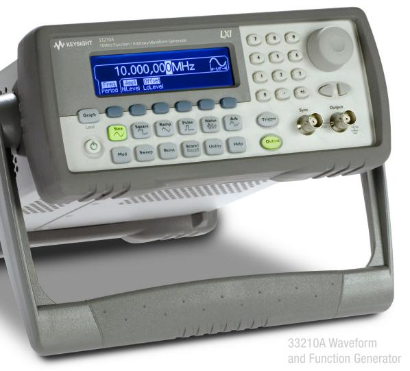
The Keysight 33210A waveform and function generator brings uncompromising performance to an entry-level instrument. Get all the basic functions and waveforms with the most stable, lowest distortion function generator in its class. The 33210A can generate primary waveforms, and an optional upgrade is available so you can generate 8 K points of complex arbitrary waveforms.
