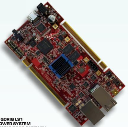
● GORIG LS1 TOWER SYSTEM MODULE FOR GATEWAY DESIGNS (TWR-LS1021A)
