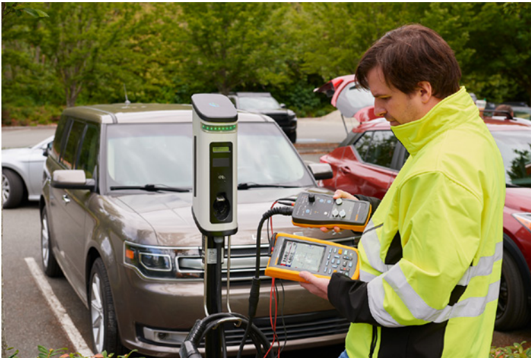
A technician can use the FEV100 with other tools, like portable oscilloscopes and power quality testers, to check out a charging station and identify common issues as part of a preventive maintenance program.
