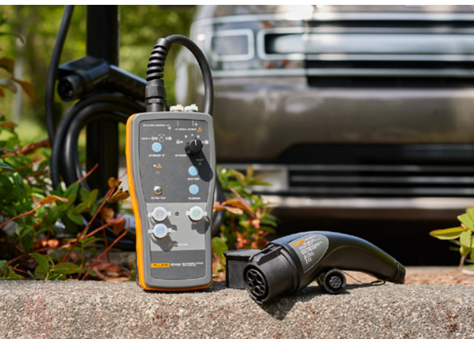
The Fluke FEV100 lets a technician test an EV charging station without an EV.
