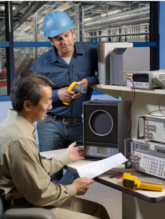
Infrared thermometers let you measure a target's surface temperature from a distance without physically touching it. To point and shoot at a target to measure its temperature may seem a little like magic. This application note demystifies the process of infrared (or "IR") thermometry and explains why regular calibration is important for maximizing the value of these useful devices.
