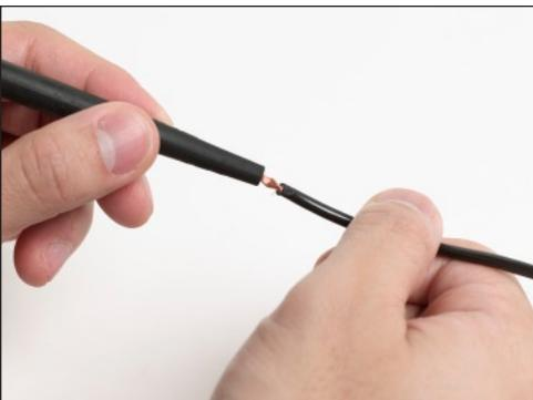
Also ensure that there are no signs of gaps or cracks at the junction between the insulated wire and the molded banana plugs or probes at each end. Though the visual inspection cannot absolutely guarantee the leads are safe, it can reveal obvious faults that can lead to injury.
