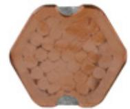
After air compression by the ABB Method, the cross section looks like this, nearly 100% metal with virtually no air spaces.
