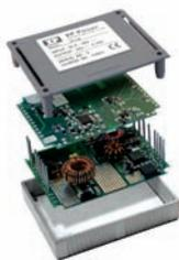
**Figure 1** – Example of 3D design technique to conserve PCB area on COTS converter.
