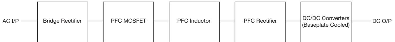
The BCC series power supply from XP is an example of a power supply designed in this way. In this instance, reliability is further enhanced by ensuring that all aluminium electrolytic capacitors are rated for operation to +105 °C and DC/DC converters with failure rates of less than 50ppm are selected.
