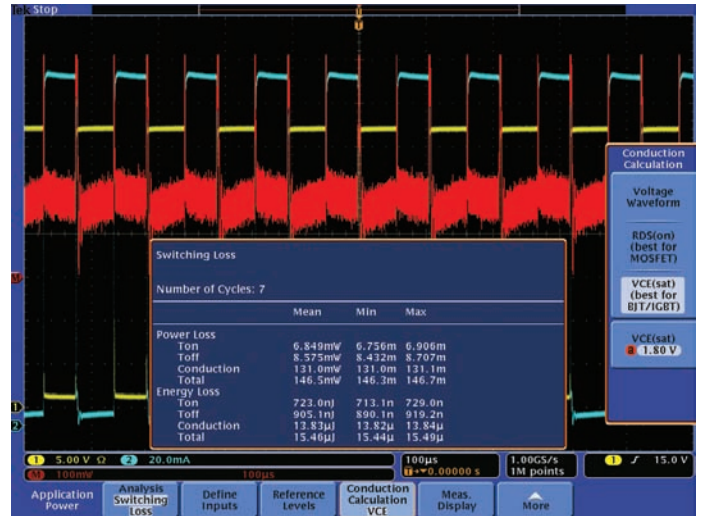
Figure 2. Switching loss measurements including statistics on the Tektronix MSO/DPO4000 Series oscilloscope and DPO4PWR power analysis software.
