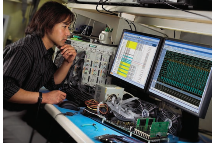
Figure 37. A complete tool set for testing energy efficient designs may include an oscilloscope, logic analyzer, real-time spectrum analyzer, time-domain reflectometer, signal generator, digital multimeter, probes and analysis software.
