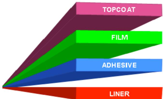
Figure 1. Construction of the high-performance labels for solar applications
