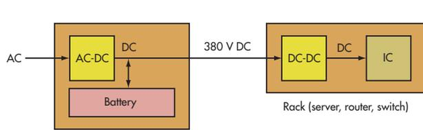
2. Using fewer conversion stages, a more efficient data-center power topology with a dc bus system and battery backup operates more efficiently, delivering 380 V dc directly to servers.
