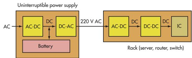
3. Somewhat efficient, a conventional data center with an ac power system employs more conversion stages.
