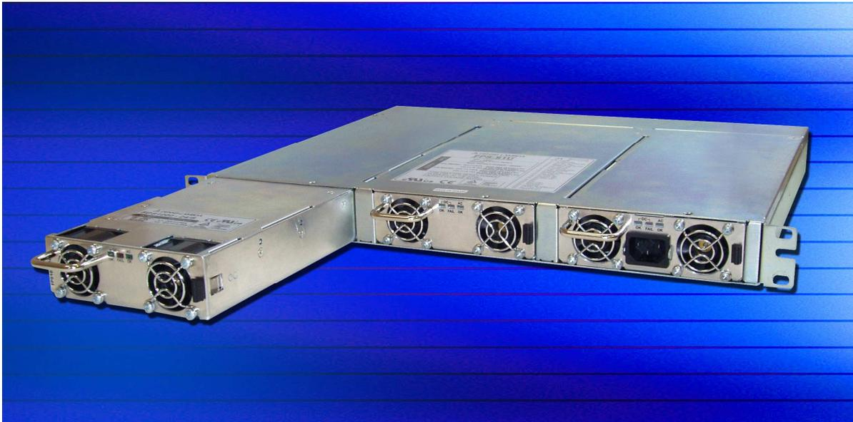
For example, TDK-Lambda’s FPS1000 Series are 1000-watt power supplies whose low profile and hot-swap capability make them especially suitable for N+1, redundant applications. The series is available with an I<sup>2</sup>C interface that monitors key functions – a requirement for remotely situated systems. Various output voltages are available including 12V, 24V, 32V, and 48V.
