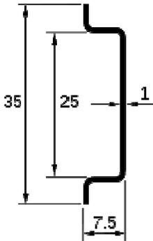
**Figure #1 – End view of typical DIN Rail**
