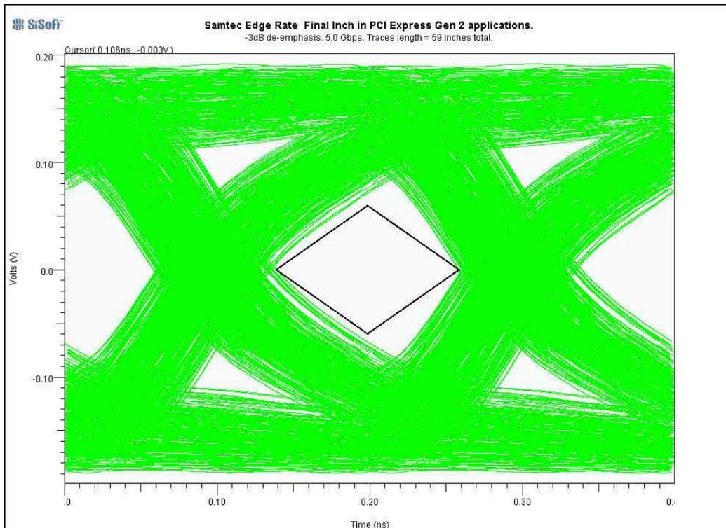
**Figure 8 – Receiver eye measurement, probed at far end termination.
