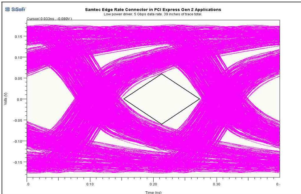
Figure 7 – Receiver eye measurement, probed at far end termination.
