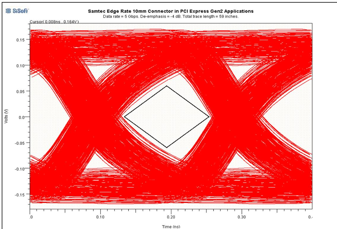
**Figure 9 – Receiver eye measurement, probed at far end termination.
