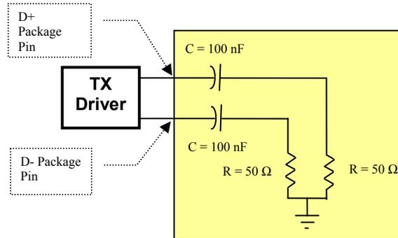
**Figure 4 - PCI Express Compliance Test/Measurement load**
