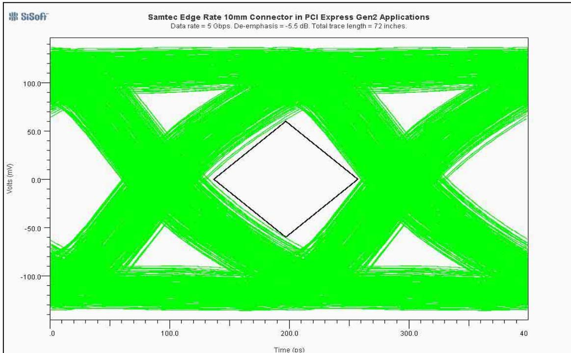
Figure 10 – Receiver eye measurement, probed at far end termination.
