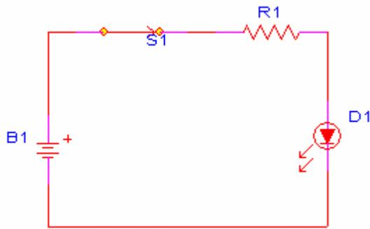
Figure 4.0: LED under test with an inrush current thermistor (R1) connected in series.
