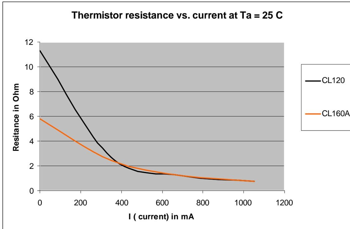
Figure 6.0: Resistance vs. current of the CL120 and CL160A (typ.)
