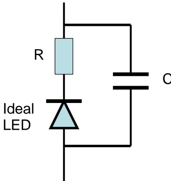
Figure 1.0: Electrical Model for a LED
