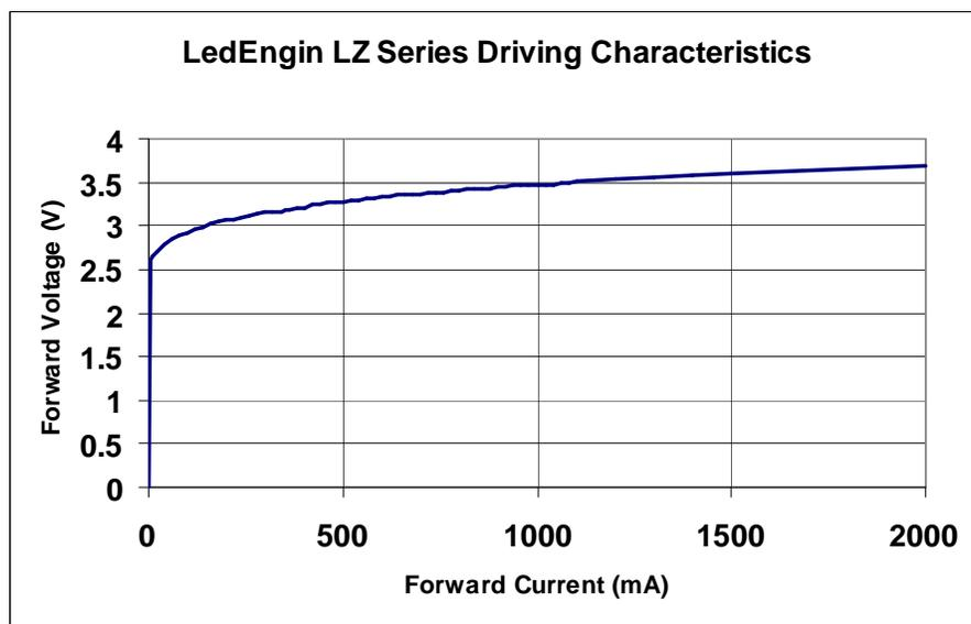
Figure 2.0: Driving characteristics of LedEngin LZ Series LEDs
