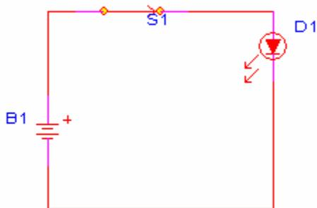
Figure 5.0: LED under test without an inrush current thermistor
