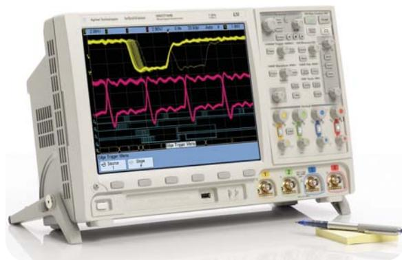
**Figure 3.** An Agilent MSO7104B quickly captures the infrequent metastable state on channel 1 while also using logic channels.
