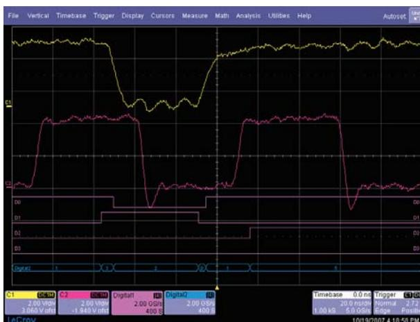
**Figure 5. The LeCroy WaveRunner 104Xi – MS500 fails to capture the infrequent metastable state after 5 seconds of observation time.**
