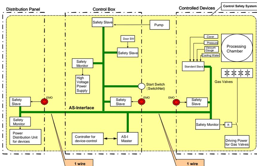
(b-1) System configuration using AS-Interface Safety at Work
