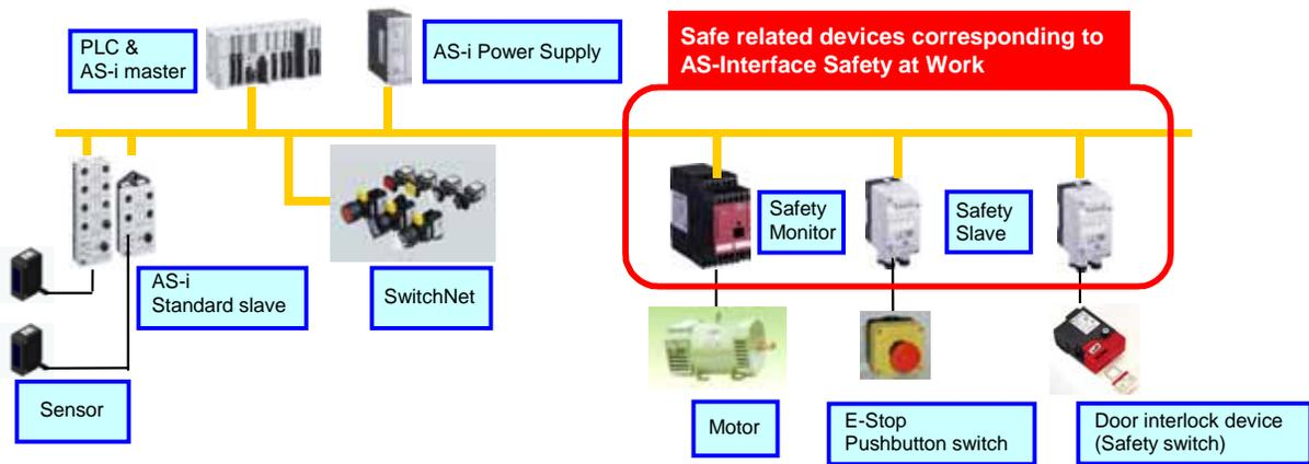
Figure 5. AS-Interface Safety at Work Basic Configuration
