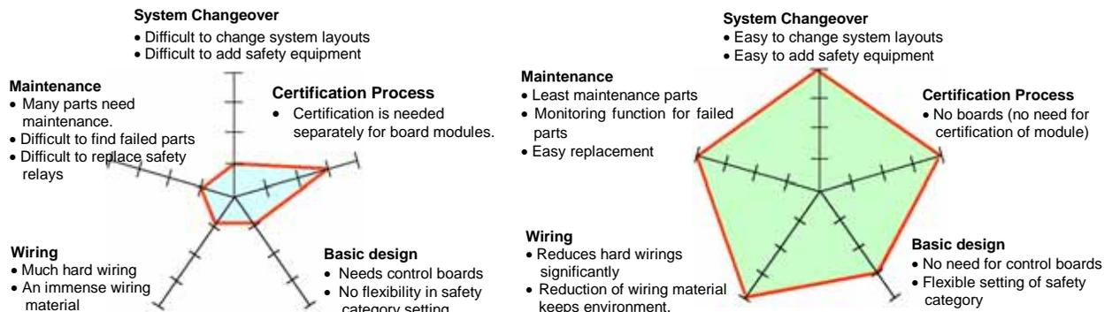
(a) Conventional Safety-related Control System (b) New Safety-related Control System using AS-Interface Safety at Work
