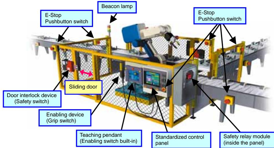
Figure 2. Model of the Manufacturing system with Robots
