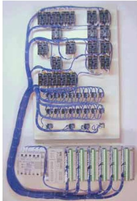
(b) Field-end components connected by the conventional wiring
