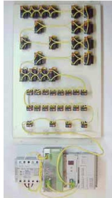
(c) Field-end components connected by the wiring of SwitchNet
