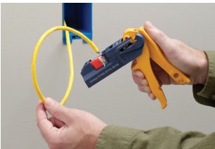
3. Insert jack in JackRapid front first with IDC slots facing blades of JackRapid.
