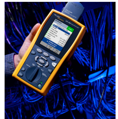
Figure 1. Certification tools take very precise measurements on parameters spelled out in TIA and ISO standards. Documented results from a high-accuracy certification tool is often the only means of meeting the requirements of manufacturers' warranties.
