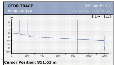
Figure 1. Depiction of a typical OTDR trace.
