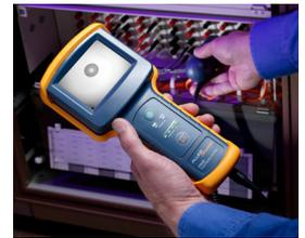
*End-face inspection, using either a handheld optical or video microscope (shown here), should be done both during and after termination to check for contaminated or improperly polished connector end-faces.*
