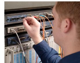
*The primary cause of fiber failures is dirty connections. Using swabs designed and sized to clean inside ports will clean an often overlooked problem source.*
