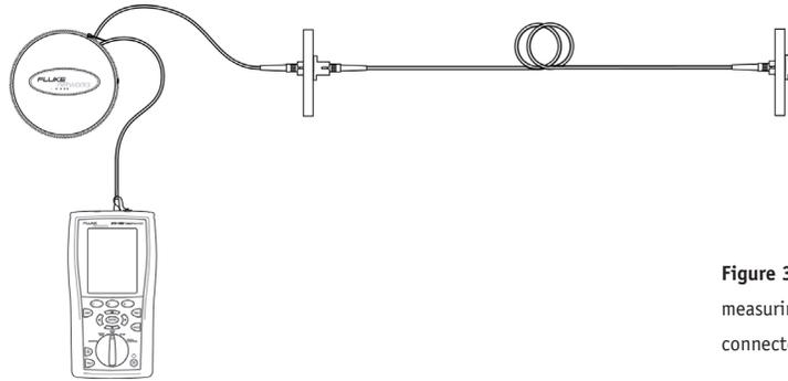
**Figure 3:** An OTDR is a single-ended test, measuring the light loss at every splice and connector on a link.
