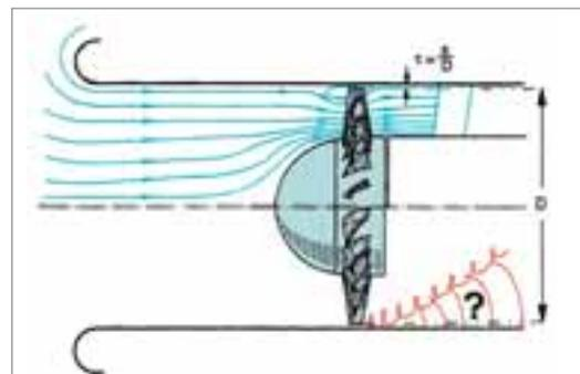
Fig. 1: Schematic flow diagram with generation of turbulence at the annular gap by difference in pressure
