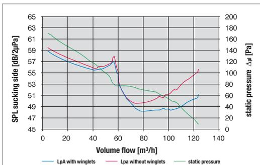
Fig. 3: Evidence that the winglets reduce the suction noise by up to 4 db(A)
