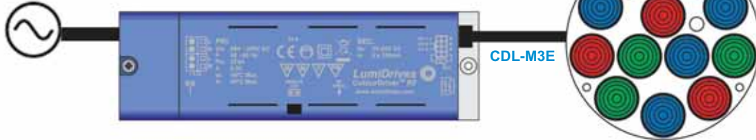
Typical Connection - With Color Engine 12
