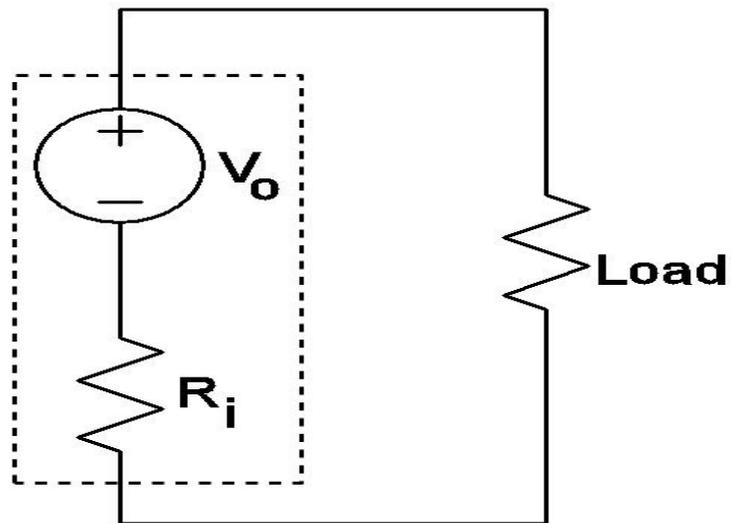
Figure 8. Circuit Model of Battery and Internal Resistance
