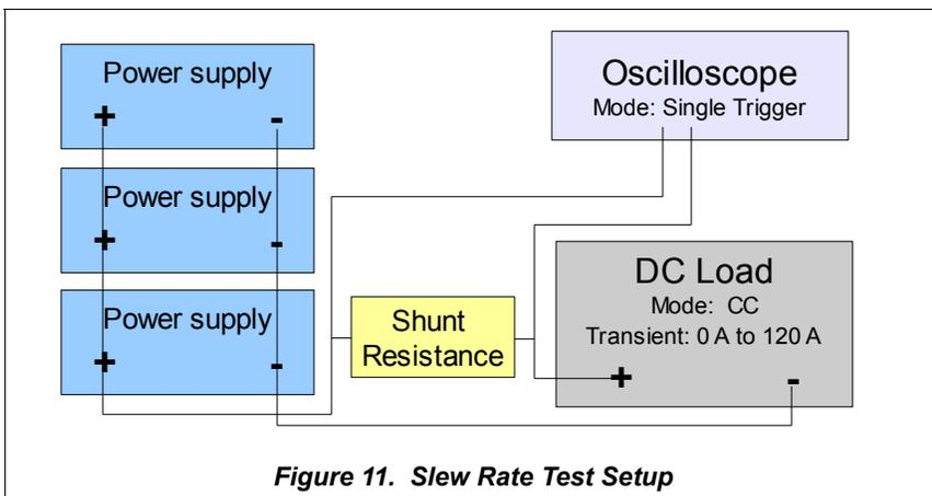
**Figure 11. Slew Rate Test Setup**
