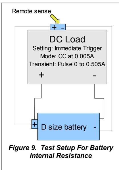
series with a resistance captures the first order behavior (see Figure 8). More complex models have also been used. Using DC loads like B&K Precision's 8500 series, batteries can be characterized in a manner which will mirror their application and construct a model appropriate for the design.
