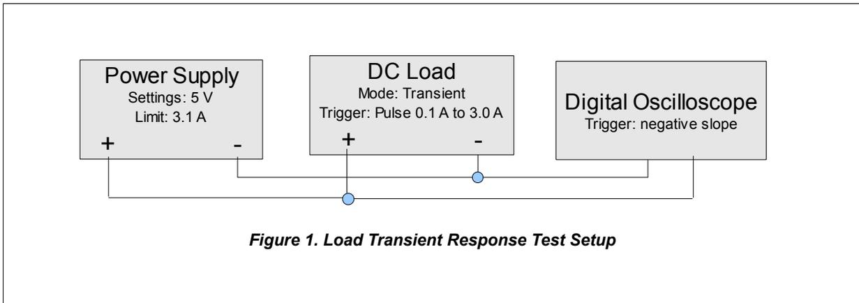
Figure 1. Load Transient Response Test Setup
