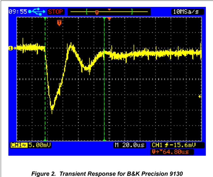
Figure 2. Transient Response for B&K Precision 9130
