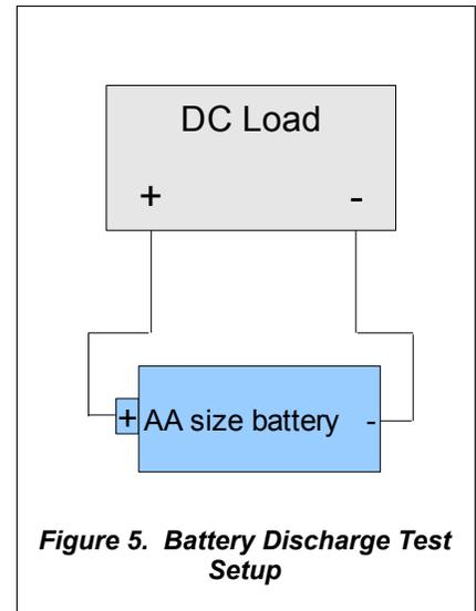
Figure 5. Battery Discharge Test Setup
