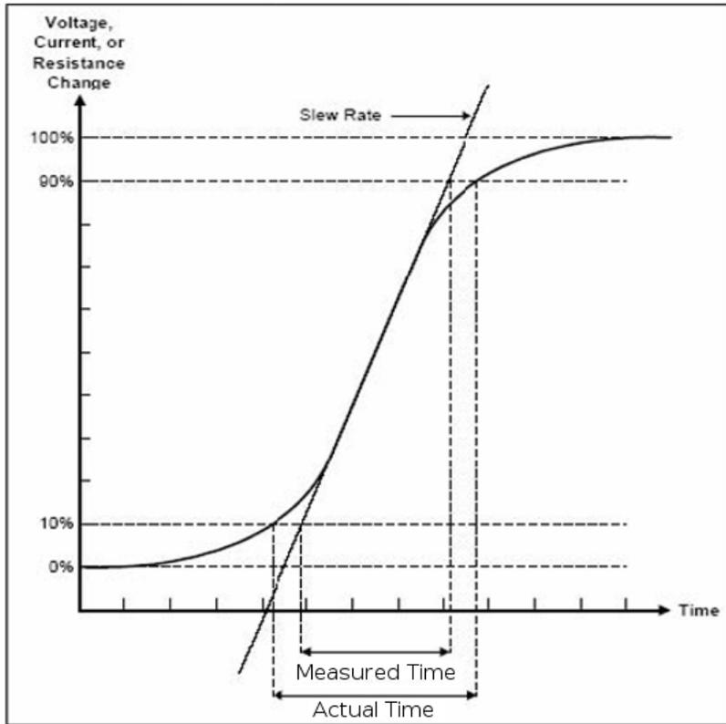
**Figure 10. Slew Rate Measurement Graph**
