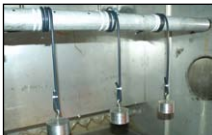
After the cold box, the cables were partially wound around a mandrel and subjected to the tension experienced through the use of an aluminum weight.
