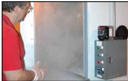
In the cold bend test, the cables were first placed into a cold box.
