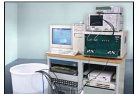
The water bath test is a six-month long test, with the cables fully submerged in water.
