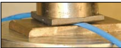
The COTS cable is smashed flat and fails at 400 lbs.
