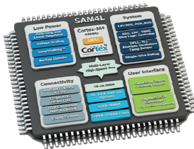
Figure 1. Block diagram of Atmel's SAM4L microcontroller.
