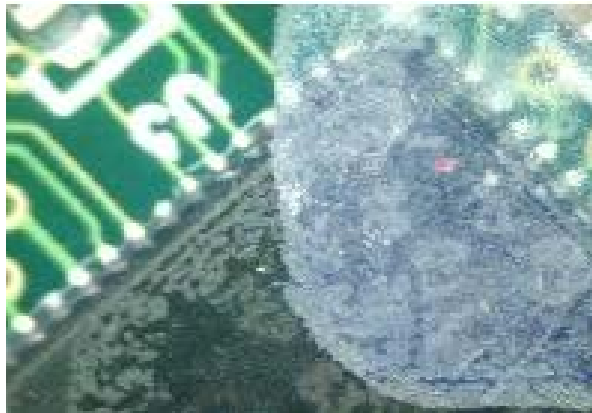
Release agents causing delamination/adhesion issue (photo courtesy of NPL)
