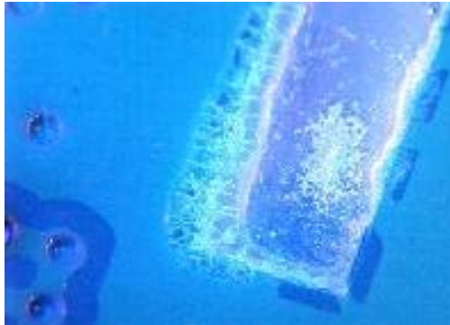
Flux residues causing coating uplift (photo courtesy of NPL)
