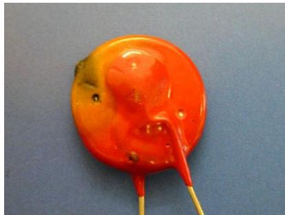
**Figure 6c: Thermally Self-Protected MOV**
