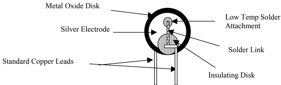
**Figure 4: Basic Construction of TMOV™ Varistor**
