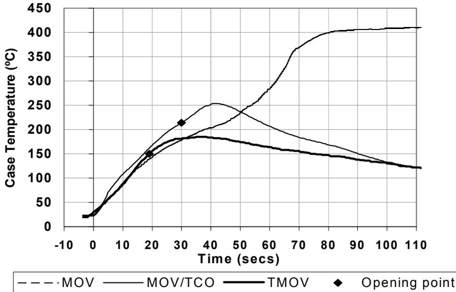
**Figure 5. Surface Temperature vs. Time for Several Protection Schemes**
