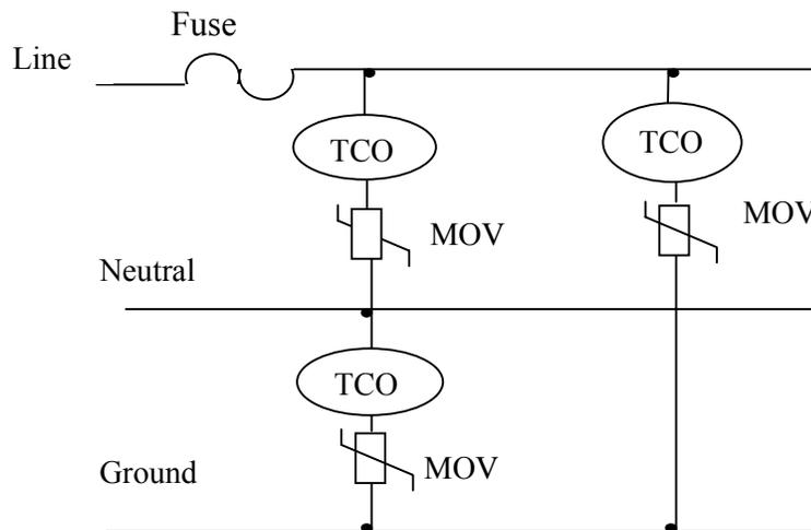
**Figure 2. Typical Off-Line Protection Scheme**
