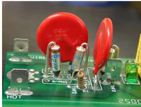
**Figure 3: Typical Arrangement of TCOs with MOVs.**
