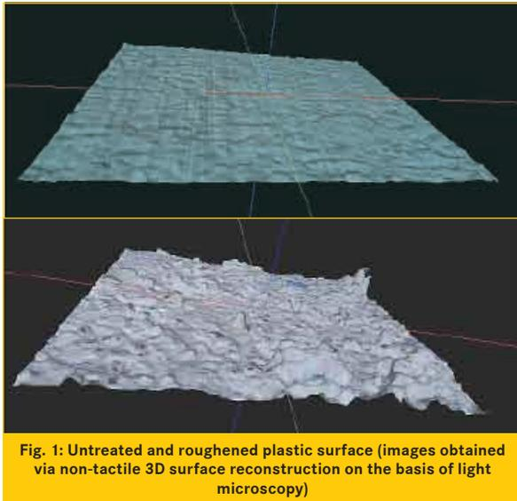
Fig.1 shows the difference between the untreated and the roughened surface. After being bombarded with particles, the surface is much rougher and this results in the optimum bonding of the zinc layer applied with the plastic surface. The resulting adhesion is 3-5 N/mm<sup>2</sup>, which corresponds to UL 746C.
