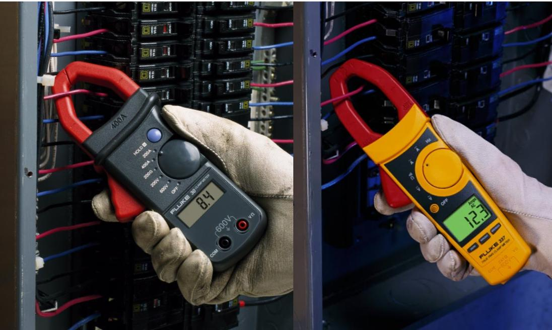
**Figure 1.** One current—two readings. Which do you trust? The branch circuit above feeds a non-linear load with distorted current. The true-rms clamp reads correctly but the average responding clamp reads low by 32 percent.
