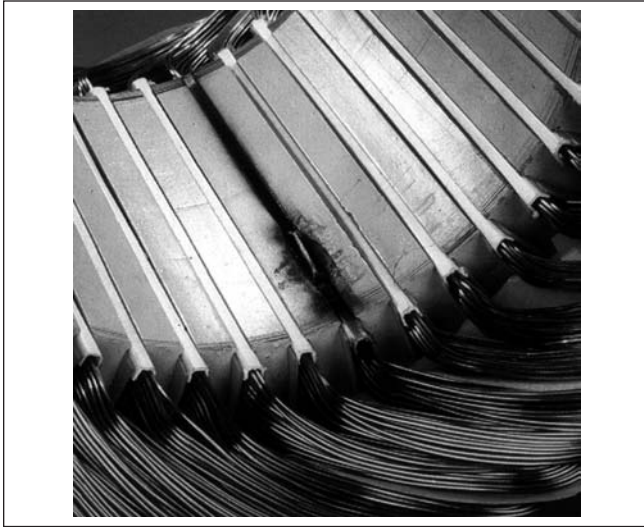
Figure 6. Example of Motor Damage Due to Ground Fault
