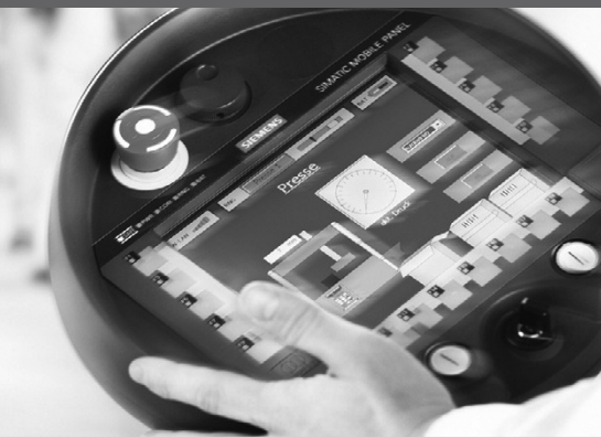
An E-Stop must be initiated by a single human action using a manual control device.
