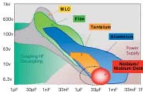
Figure 2. Technology CV Diagram.
