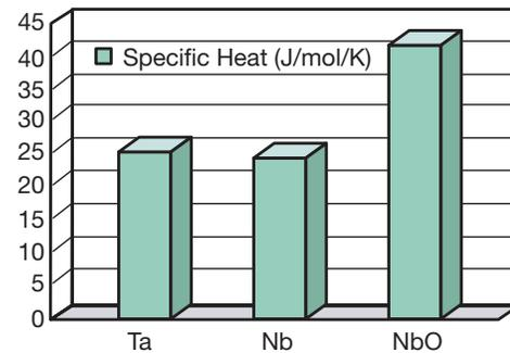
Figure 6, 7. Comparison of Ignition Rate, Ignition Energy and Specific Heat for NbO, Ta and Nb metal powders.
