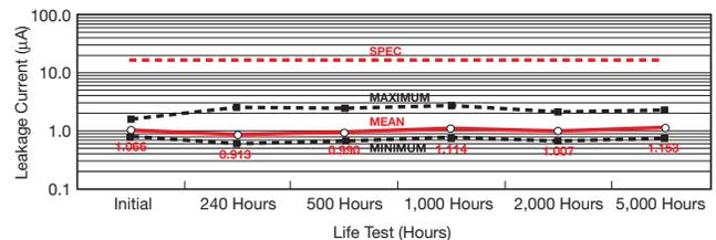
Figure 3. Leakage Current Stability on 85°C Life for 5,000 hours.
