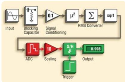
Figure 1. Block diagram of an analog AC converter
