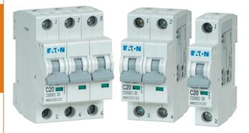
Eaton's WMZS line of miniature circuit breakers includes a broad range of devices defined as "supplementary protectors." These breakers comply with UL® 1077 and CSA® 22.2 No. 235 regulations defining supplementary overcurrent protection. In these applications, branch circuit protection is not required, or is provided by a separate device like a fuse or molded case circuit breaker.
