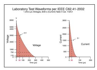
**Figure 1.** Because this generation has an internal impedance of  $20\Omega$ . The peak current value will be 3000A. The suppressor is connected to the generator for testing.
