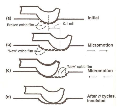
Figure 5. Fretting corrosion from micromotions
