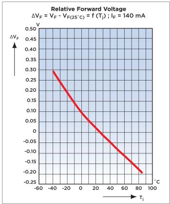
Figure 2. Forward voltage drops as junction temperature rises.
