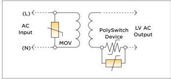
Figure 5. A coordinated protection scheme for Class 2 power sources.
