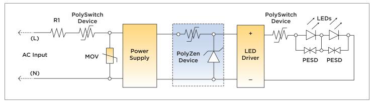
Figure 4. Coordinated protection scheme for LED Driver inputs and outputs.
