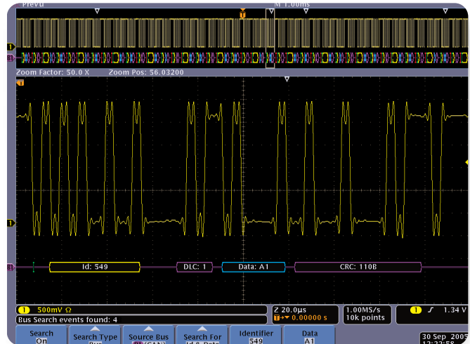
► Figure 18. Searching on specified Identifier and Data in a CAN bus acquisition.
