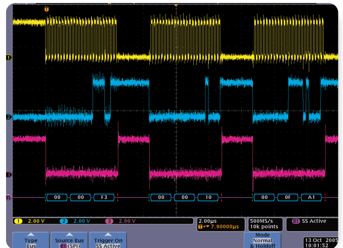
► Figure 13. Correct synthesizer configuration messages.
