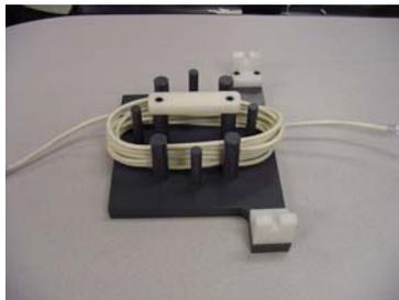
Patch Cord compressed into a 2.5-inch coil to form an ellipse
