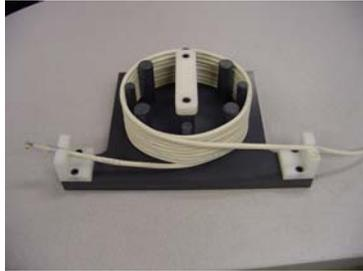
Patch Cord put into a 6-inch diameter cable loop, up to 10 loops total
