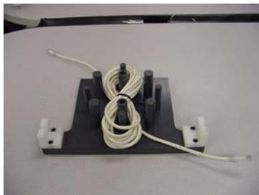
Patch Cord rotated on one end on the coil ellipse by 180° to form a figure eight
