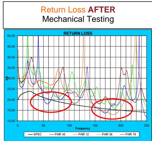
TIA/EIA 568-B.2 mechanical stress test of high quality patch cords, such as the *PANDUIT® TX6™* Patch Cords shows electrical performance that exceeds the TIA/EIA 568-B.2 specifications resulting in **superior long-term channel performance and increased network reliability.**
