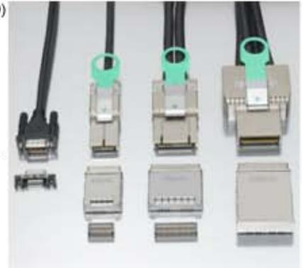
Molex's full range of connectors and cables include a high durability x1 TDP™ (rated for 1500 mating cycles) and x4, x8 and x16 iPass™ configurations (rated for 250 mating cycles). Molex also provides a complete offering of PCIe test boards for testing requirements.
