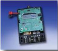
The MCP3909 and PIC18F25K20 Low Cost Power Monitor is a fully functional single phase meter. The design is intended to be low cost and uses a shunt current sensing element. A single MCP3909 acts as the analog front end measurement circuitry. The LCD module is used to display RMS current, RMS voltage, power factor and active power. The meter design is intended to be flexible and able to be upgraded to a variety of PIC microcontrollers.
