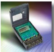
This reference design is a fully functional 3-phase energy meter including PC software used for automated calibration. The reference design consists of two boards: the main metering board with the MCP3909 devices and PIC18F2520 that performs the power calculations, and the USB interface module which uses the PIC18F4550. The meter design contains serially accessible registers and is intended to be flexible and upgraded with a variety of PIC microcontrollers using the included firmware.
