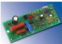
This low-cost energy meter board acts as a stand-alone energy meter or as the analog-front-end design for LCD microcontroller-based meters. The MCP3905A design is specified with an energy measurement error of 0.1% typical across 1:500 dynamic range for high accuracy energy meter designs. The board is compliant with EMC requirements per energy metering standards IEC62053 and legacy IEC61036, IEC1046 and IEC687.
