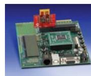
The Explorer 16 Development Board offers an economical way to evaluate Microchip's 16- and 32-bit microcontrollers, and dsPIC33F DSC Families. Developers are able to create IEEE 802.15.4™/ ZigBee and IEEE 802.11™/Wi-Fi wireless communication applications by adding wireless PICtail daughter cards to the Explorer 16 using the associated software protocol stack.
