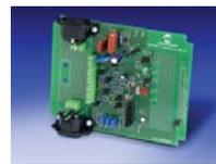
This evaluation board allows the user to test a variety of energy meter designs. On the input side, high voltage line and load AC-plug headers are included, along with mounting holes for shunts, current transformers and screw-type connections for wiring. On the output side, a large prototype area is included along with optical isolation and a standard PICtail™ header for experimenting with a variety of PIC microcontroller-based energy meter designs.
