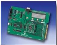
The MCP3901 ADC Evaluation Board for 16-bit MCUs provides the ability to evaluate the performance of the MCP3901 dual channel ADC. It also provides a development platform for 16-bit PIC based applications using existing 100-pin PIM systems. A LabVIEW software interface enables viewing of the MCP3901 performance via USB interface.
