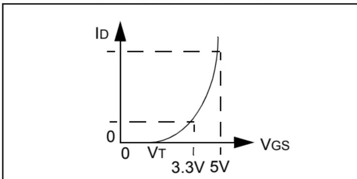
Low threshold devices commonly exist for MOSFETs with drain-to-source voltages rated below 30V. MOSFETs with drain-to-source voltages above 30V typically have higher gate thresholds (VT).
