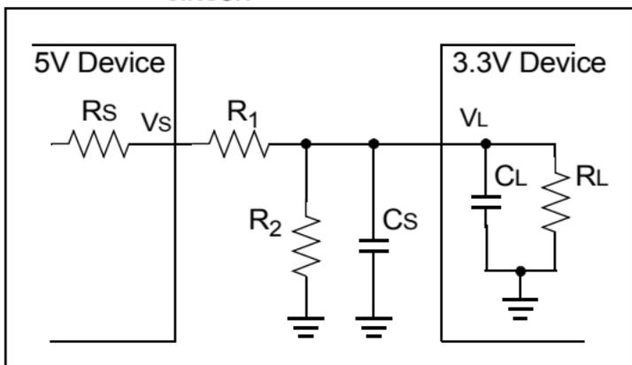
Typically, the source resistance,  $R_s$ , is very small (less than 10 ohms) so its affect on  $R_1$  will be negligible provided that  $R_1$  is chosen to be much larger than  $R_s$ . At the receive end, the load resistance,  $R_L$ , is very large (greater than 500 k ohms) so its affect on  $R_2$  will be negligible provided that  $R_2$  is chosen to be much less than  $R_L$ .
