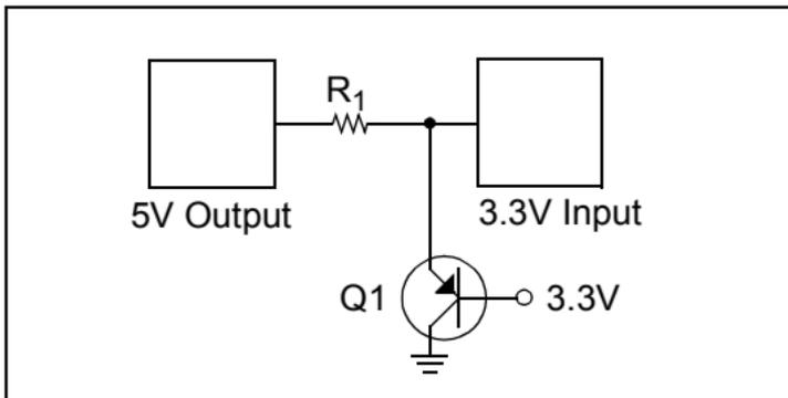
The base-emitter junction of Q1 performs the same function as the diode in a diode clamp circuit. The difference is that only a small percentage of the emitter current flows out of the base of the transistor to the 3.3V rail, the bulk of the current is routed to the collector where it passes harmlessly to ground. The ratio of base current to collector current is dictated by the current gain of the transistor, typically 10-400, depending upon which transistor is used.
