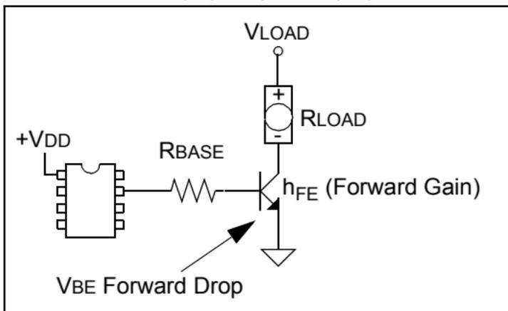
The value of  $R_{BASE}$  will depend on the microcontroller supply voltage. Equation 18-1 describes how to calculate  $R_{BASE}$ .
