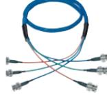
L-com's low loss (male-to-male) 75 Ohm coaxial cables are suitable for transmitting RGB video signals. Lightweight coax cables utilize spiral shielding for extra flexibility.
