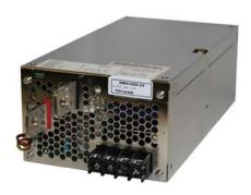
Above is a photo of an HWS series power supply that can provide 1000 watts of output power and features alarm signals and active current sharing. Two or more of these supplies can be connected in parallel with external "ORing" diodes to form a redundant and fault tolerant power system.
