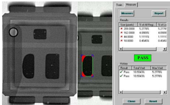
Figure 18 Poorly formed source joint – 11% missing
