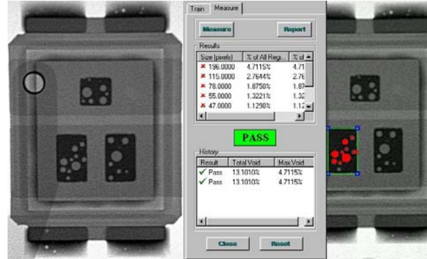
Figure 13 Voids on the left source contact
