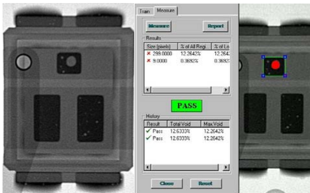
Figure 12 Voids on the gate contact
