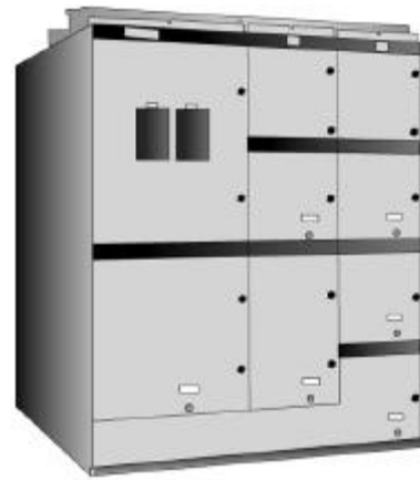
FIGURE 5: TYPICAL LOW VOLTAGE METAL-ENCLOSED ASSEMBLY
