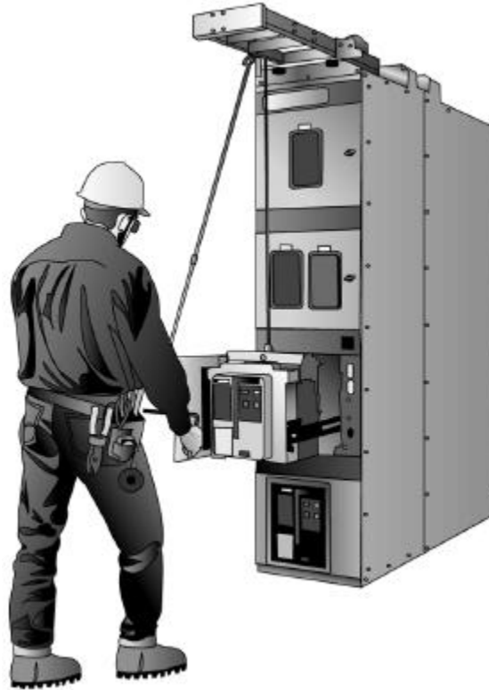
FIGURE 29: RAIL MOUNTED LIFTING DEVICE BEING USED TO LIFT A MAGNUM DS POWER CIRCUIT BREAKER FROM ITS COMPARTMENT EXTENSION RAILS
