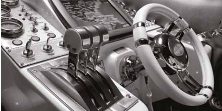
The choice of material and resistance to saltwater corrosion is important in marine applications. Above right: EAO Series 14 with silicone lens cover
